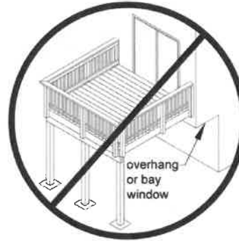
Figure 18. No Attachment to House Overhang with Ledger.
