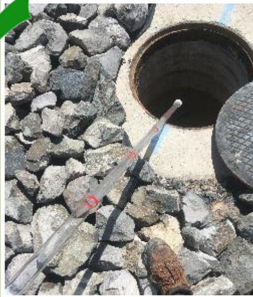
Use a “sludge judge” or similar to check for sediment in a separator’s sump
