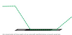
An example of the path of an aircraft performing a touch and go.
